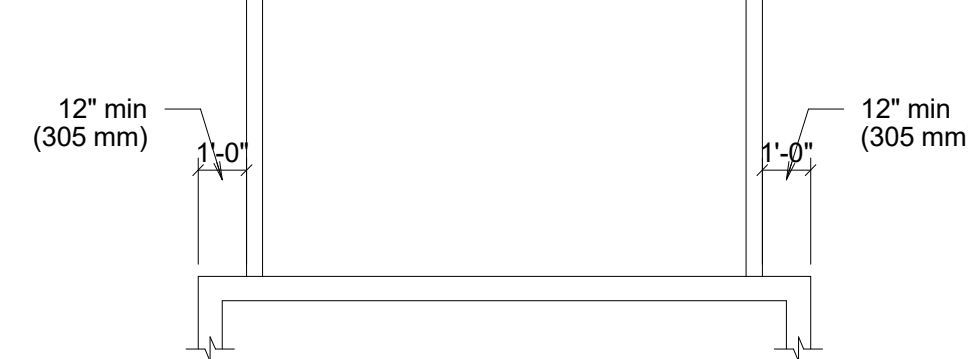
Figure 405.9.1 Extended Floor or Ground Surface Edge Protection
